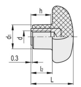
$\begin{array}{lll} D & = 40 \\ D1 & = 16 \\ DH & = M6 \\ h & = 13 \\ I2 & = 13.5 \\ L & = 27 \\ Weight in (g) = 24 \end{array}$
